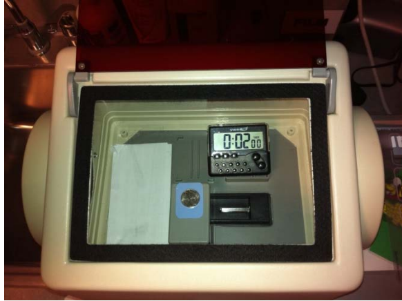
Figure 1 – Intraoral Fog Test Set-up in a Glove box
